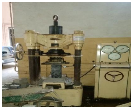
Figure 1.0: Column Test Setup
