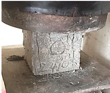
Figure 6. Crack patten at compressive failure of Specimen CL-40
